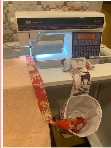
**Method 2:** Roll the binding into a spiral, then place it on the upright thread spindle of your machine to have it unroll smoothly.
