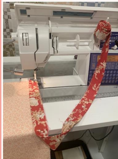
**Method 3:** Wind the binding around an empty thread spool, loop a ribbon through the spool and suspend it from a drawer handle so it will unroll smoothly as you sew.
